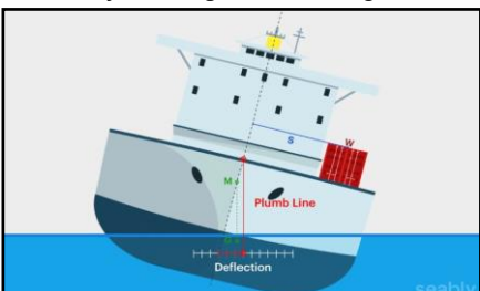
Inclining test / architectural assessment
